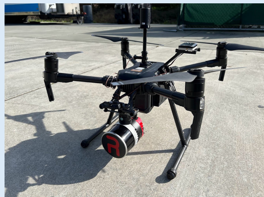
Fig. 2: DJI Matrice 200 Quadcopter with RESEPI XT-32 LiDAR
